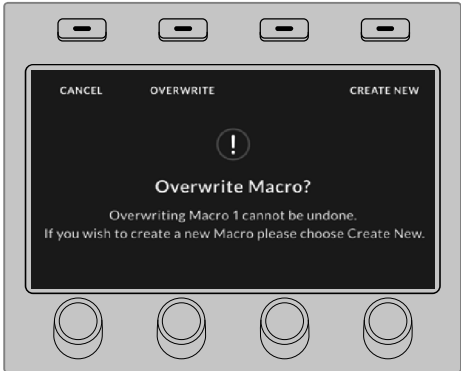
If you want to record over a previously recorded macro, or if you made a mistake and want to start recording the macro again, press the record button and confirm the overwrite when prompted.
